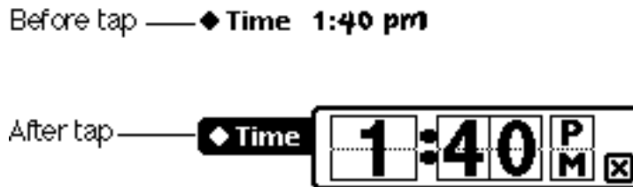
Figure 5-20 Example of a label picker with a text representation of a time delta
