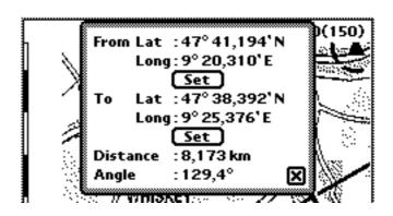
The calculator will need two reference positions which you can enter while this window is open. After entering the first position tap onto the upper **Set** button and the reference position will be displayed. Then define the second reference position and press the lower **Set** button. The calculator will show the second reference position and the distance and course (geographic north relative) between both positions.
