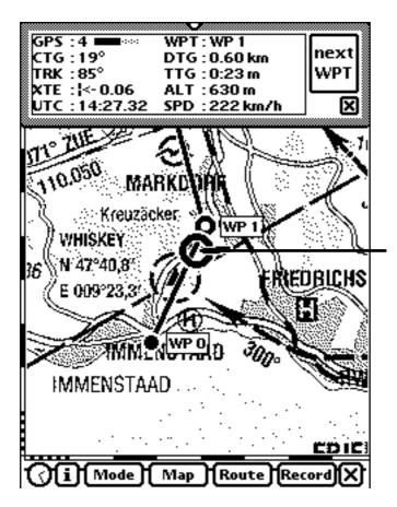
the actual position is at the center of the circle, the pointer shows to the movement direction
