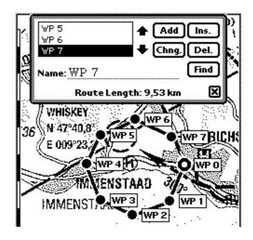
If a route is loaded its way points will be displayed in the list. To enter a new way point first define a reference position for the waypoint and then tap Add for appending the new waypoint or Ins. for inserting the way point before the way point currently selected in the list.
