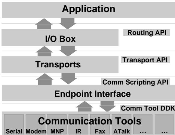
Figure 1: Newton Communications Layers
