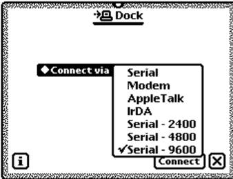
In the *Dock* slip on the Newton, tap 'Connect Via' and select 'Serial- 9600' to connect to Win 3.1 or Win95.
