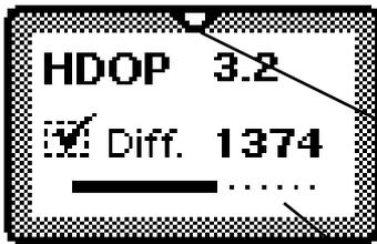
*When you are collecting real time Differential GPS, this floater will appear on the screen. If you want to move it, hold your pen down on the hanger and slide it to a better place on the screen.*
