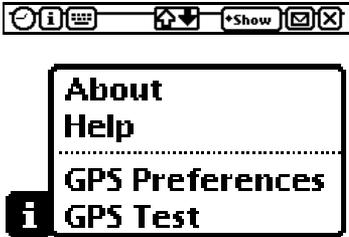
Because GPS receiver settings apply to all projects, access to GPS settings is contained in the 'i' button at the bottom of the screen. The context sensitive help is also contained in the button because it is always available.
